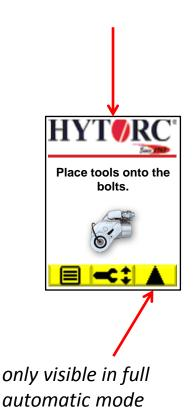
19) In case of *Stop* was pressed, the motor is off and the system waits to resume operation.
