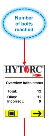
43) *Trigger* is released and the motor is off. An overview of the bolts status is displayed.
