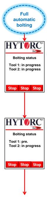
38) **Trigger** is pressed, the pump starts the full automatic process and the current status of each bolt is displayed on the fly. In case of active pre-tightening and more than one tool is connected, the pump is going to pre-tighten the bolts to a low torque level depending of type and size of the tools. Still hold the **Trigger**.
