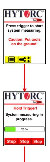
33) Press and hold the *Trigger* to start system measuring. Caution: Put tools on the ground!
