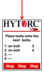
42) *Trigger* is released, the full automatic process is finished. Now you can place the tools onto the next two bolts.
