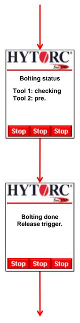
40) *Trigger* is pressed, one bolt is tightened and is marked as "checking". If all bolts are tightened, the pump will start to run the control strokes.
