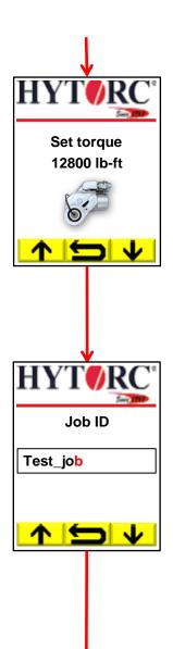
24) Set the required torque for the bolting job.
