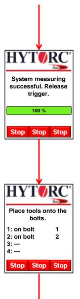
35) System measuring is complete and an acoustic signal sounds. Please release the *Trigger*.
