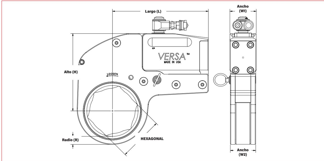
LEYENDA: H = ALTURA W1 = ANCHO DEL CABEZAL W2 = ANCHO DEL ENLACE L = LARGO R = DISTANCIA DESDE LA ESQUINA HEXAGONAL
