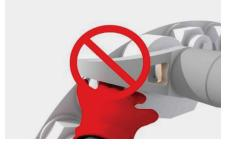
The J-Washer provides outer reaction lobes that safely engage with a socket driver or reaction plate to brace the reaction forces during torque operations. Consistent with the standard HYTORC Reaction Washer, the new J-Washer eliminates the need for a separate reaction arm, eliminating pinch points and significantly reducing the risk of hand injury.
