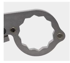
The high strength steel backup wrench is suited for heavy duty industrial bolting applications. The Backup Wrench comes in a range of sizes with 12-point cutouts so that it can be matched to the specific bolting job.
