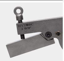
The Backup Wrench is provided with an adjustable arm that simplifies installation in a variety of configurations. The eye-bolt on the arm may be adjusted to quickly to lock the wrench in place or to unlock following the bolting operation. Add a lanyard to the eye-bolt to prevent drop hazards.
