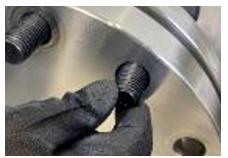
Install the bolt through the bolt holes allowing enough length on the front side for the nut, Reaction Washer and 2 to 3 extra threads.
