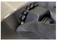
Tighten the nut by hand until snug.
