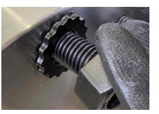
Verify that the nut will run free by hand onto the bolt on the front of the flange.
