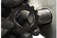
Ensure the HYTORC J-Washer is installed with the beveled side containing outer knurl ridge faces the flange and the flat side containing inner knurled ridge faces the nut.
