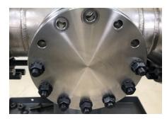
Align flanges per PCC-1 requirements and ensure fastener surfaces are free of defects.
