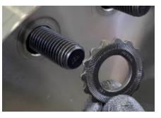
Align the HYTORC Reaction Washer or J-Washer with the bolt on the front side of the flange.
