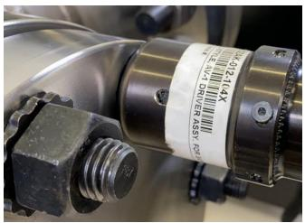
Position the socket over the nut and washer. Make sure the driver is fully engaged on the hardware and tighten to specification.
