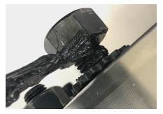
Apply lubricant to the nut spot face.
