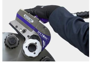
Position the link over the nut and washer. Make sure the link is fully engaged on the hardware and tighten to Specification.
