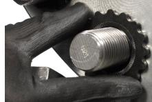
Install the Reaction Washer or J-Washer over the bolt with beveled side facing the flange and the flat side facing the nut.
