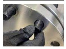
Install the bolt through the bolt holes allowing enough length on the front side for the nut, Reaction Washer and 2 to 3 extra threads.
