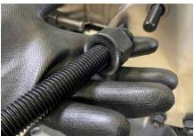
Inspect bolts, nuts and washers to ensure they are free defects that would prevent proper assembly.
