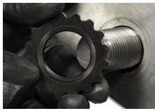
Ensure the HYTORC J-Washer is installed with the beveled side containing outer knurl ridge faces the flange and the flat side containing inner knurled ridge faces the nut.
