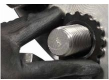
Verify that the nut will run free by hand onto the bolt on the front of the flange.
