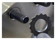
Ensure the HYTORC Reaction Washer is oriented with the beveled knurled side facing the flange and the smooth flat side facing the nut.
