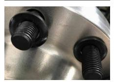
Install the HYTORC Backup Washer over the bolt on the rear of the flange.
