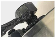
Apply lubricant to the nut spot face.
