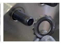
Align the HYTORC Reaction Washer or J-Washer with the bolt on the front side of the flange.
