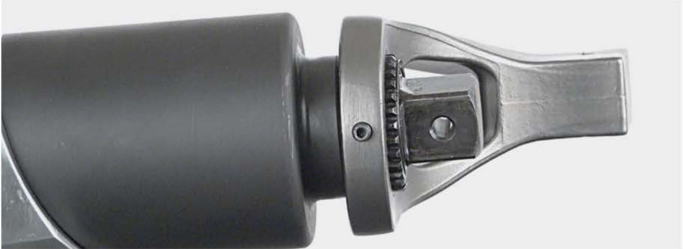
1. FLAT ON REACTION SPLINE. 2. ALLEN SET SCREW
