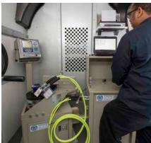
Our mobile calibration lab provides on-site calibration of manual torque wrenches as well as hydraulic, pneumatic and electric tools with torque output up to 20,000 ft-lbs. For calibration of larger tools, our service technicians offer pickup and drop-off service.
