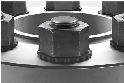
The HYTORC Washer eliminates the need for reaction arms, which are the most common cause of injury on bolting jobs. The unique design of the washer allows the double layered safety socket to react on the washer itself, while turning the nut.
