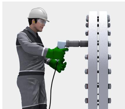
No pinch hazards; intuitive operation; less personnel; no damaging side loads or bending forces; nuts and bolts can be reused.
