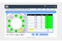
The App remains wirelessly connected to the tool during bolting operations to guide the operator to successive lugs and bolts. The App provides immediate confirmation after each tightening operation and alerts the operator if there is a need to repeat a task to meet specifications. The App provides graphical instructions until tasks are complete to ensure all bolts are tightened properly.
