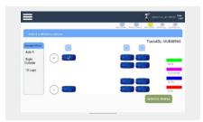
The Fleet App offers a simplified method for configuring vehicles, bolting patterns, sequences and torque specifications. The user enters all vehicle configuration and bolting setup parameters conveniently on the tablet. The App is quickly connected to the electric tool via Bluetooth<sup>®</sup> Wireless Technology and all setup and configuration data is automatically sent to the tool avoiding any input errors.
