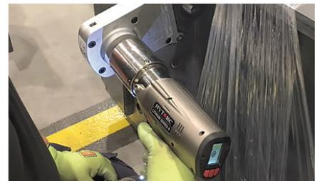
The Offset Link provides an interchangeable cartridge system that allows the user to easily change out cartridges in the field to accommodate a range of hex sizes. The Offset Link is compatible with the HYTORC Washer which eliminates bending and side load while increasing the safety and speed of all bolting operations.
