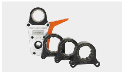
The Offset Link is compatible with all HYTORC Hydraulic, Pneumatic and Electric Torque tools. The Offset Link comes in two basic drive types compatible with either  $\frac{3}{4}$ " and 1" square drives. The torque multiplication factor for each cartridge is clearly marked; simply multiply the factor by the desired torque and set the torque on the tool for accurate and repeatable bolting operations.
