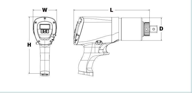
**LEGEND: H** = HEIGHT **W** = WIDTH **L** = LENGTH **D** = OUTER DIAMETER OF GEARBOX
