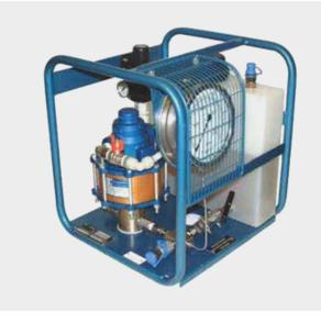
This easy to use, air-driven hydraulic pump is mounted in a tubular steel transportable frame painted blue. The pack is supplied complete with, air inlet connector, air filter, air pressure regulator, air lubricator, air pressure gauge, air pressure limit valve, pump on/off control, oil reservoir, oil pressure release valve, oil pressure gauge, gauge guard, air/hydraulic pump and high pressure oil outlet through a self sealing quick connect coupling.
