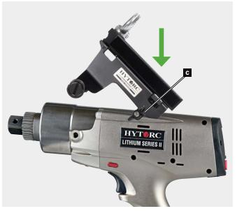
STEP 1: Position the LST Tool Hanger over the tool as shown. Align locating pin (C) with the tool's insert hole. Slide locating pin firmly into hole.
