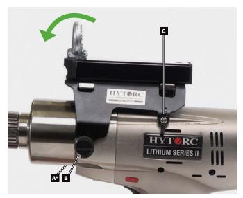
STEP 2: Pivot down the LST Tool Hanger so captive screws (A) and (B) align with the tapped holes on both sides of the tool. Hand-tighten both captive screws and the wing nut on locating pin (C) until fully secured. adjust the sliding beam (E) to the desired position. Take caution not to cross threads.
