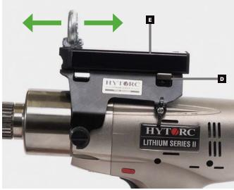
STEP 3: The adjustable eyelet allows better balance of the tool when equipped with various sockets and reaction arms. Push down the thumb lever (D) and
