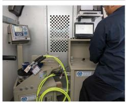
Our mobile calibration lab provides on-site calibration of manual torque wrenches as well as hydraulic, pneumatic and electric tools with torque output up to 20,000 ft-lbs. For calibration of larger tools, our service technicians offer pickup and drop-off service.
