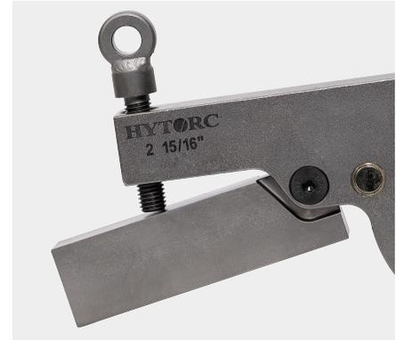
The Backup Wrench is provided with an adjustable arm that simplifies installation in a variety of configurations. The eye-bolt on the arm may be adjusted to quickly lock the wrench in place or to unlock following the bolting operation. Add a lanyard to the eye-bolt to prevent drop hazards.
