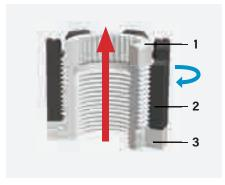
The HYTORC Nut is composed of an inner sleeve, outer sleeve, and washer. As the outer sleeve turns (blue arrow), the inner sleeve moves upwards (red arrow).
