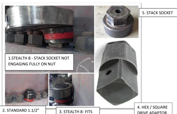
70MM SOCKET FITS IN BETWEEN BOLTS AND ENGAGES FULLY
