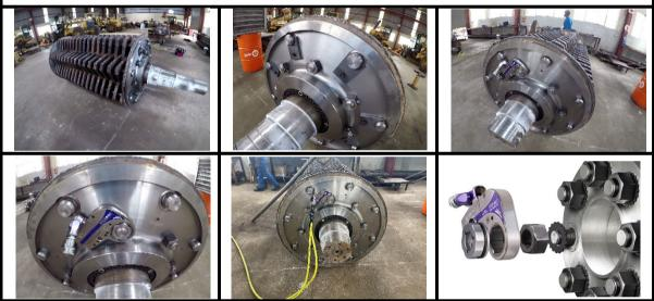
**SOLUTION**: HYTORC visited the facility and demonstrated the use of Stealth and Avanti tools for the application, the tools were powered by Vector pump, Customer initially had a high torque value and were not using lubrication. This was added and a recommended torque value was agreed upon. The bolts have Standard nuts and utilise split pins to secure the bolts after tightening, HYTORC propose to use back up waashers with long-term goal of utilising HYTORC reaction washer.
