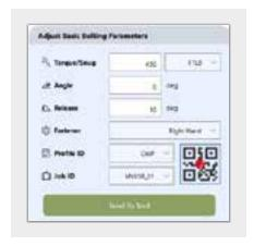
To reduce the possibility of errors, the HYTORC Connect App enables the user to easily type or scan QR codes with job parameters, and send them automatically to the tool.
