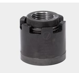
The CT-Series Nut's thicker outer sleeve minimizes stress and allows it to handle high loads at elevated temperatures. The through-bolt design makes them ideal for applications with high stud protrusions from the flange.
