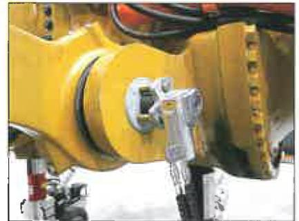
**ICE Bolting System with 797 Collett Bolt Fixture**
