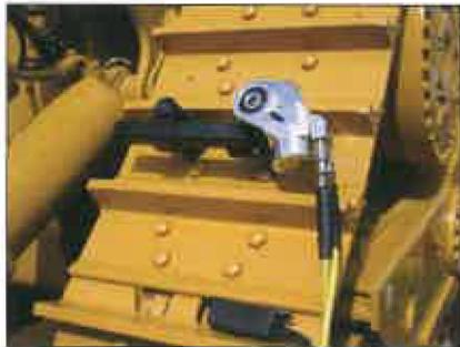
**Avanti Bolting System with Safety-Enhancing Track Fixture**
